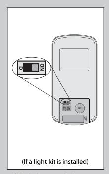
If a light kit is installed on your fan, choose the light bulb mode by moving the toggle switch.
