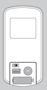
To change the battery, remove the battery door. Remove battery and replace with A23 or MN21 alkaline battery. Please observe proper polarity placement.
