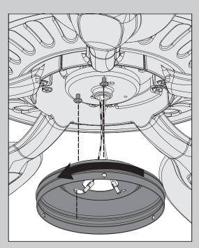
Feed the optional light kit wires through the center hole of the upper switch housing, then wrap keyhole slots around the screws and twist counterclockwise.
