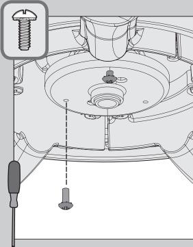
Screw two housing assembly screws from the ≡ hardware bag halfway into the mounting plate. It does not matter which two screw holes you choose.
