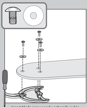
Insert blade screws and washers found in the A hardware bag into the holes in the blades, then secure each blade to a blade iron.
