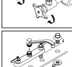
(2) Install spout to the faucet body. Place the faucet through the mounting surface. Slide the crowfoot washer through shank from underneath of the mounting surface. Tighten the locknut with the help of 1-3/32" socket set. For a faucet with a side spray, place side spray holder on mounting hole. Tighten locknut from underneath the sink to secure the side spray holder.
