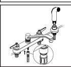
(4) Guide the side spray hose through the side spray holder. Insert the side spray hose quick connect adapter into faucet outlet end, push until a "click' is heard. Pull side spray hose downward to test engagement.
