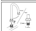
(3) For spout model number CS-22002, CS-22003, utilize friction brass washer to make spout rigid by removing Nylon gasket and replacing with friction brass washer, tighten retainer nut to the faucet body with wrench.
