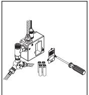
(6) Use screw driver to take out battery cover plate and put 4x AA batteries into compartment. Secure the battery cover back to module. (Note: Perform this step only if hands are dry.)
