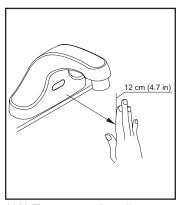
(10) To set sensing distance: Press and hold ON/OFF button for 5 ~ 7 seconds. When the LED sensor light remains lit, the system has entered setup mode. Place an object, or your hand, at desired distance. Note that the LED sensor light should be flashing when object is detected. To set the new distance, press the ON/OFF button again, your settings have been saved.
