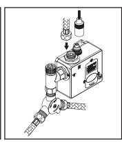
(5) Connect hose and sensor plug from faucet to control module. (Note: Do not connect sensor cables when hands are wet.)
