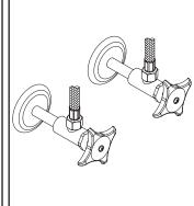
(4) Connect inlet hoses to angle stops.
