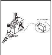
(7) Plug AC adapter to the bottom of the control module. (Note: For -AC variations.) (Note: Perform this step only if hands are dry.)
