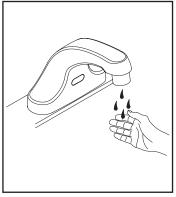
(9) Factory preset sensing distance is 12 cm (~4.7 in), please place an object or hand at about this distance and let water flush any debris from supply line for at leas one minute. Put aerator back to spout and press ON/ OFF button again.
