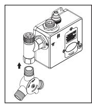
(2) Secure mixing valve onto (3) Secure inlet hoses to the control module as shown mixing valve as shown in in picture. (Note: Not for -LM picture. (Note: Not for -LM variations.)
