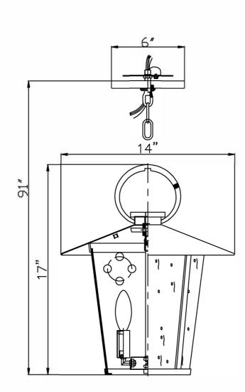
WARNING: O All electrical components must be installed by a licensed electrician in accordance with the National Electric Code and the appropriate local electrical codes. LISTED You will need 4 - Cand.Bulb 40 Watts Recommended 60 Watts Max USE LED BULBS FOR EXTENDED USE California T24 JA8-2016 Qualified: Satco (S9612); 10.5 watt LED Medium Base recommended. Bulb not included This fixture is WET rated
