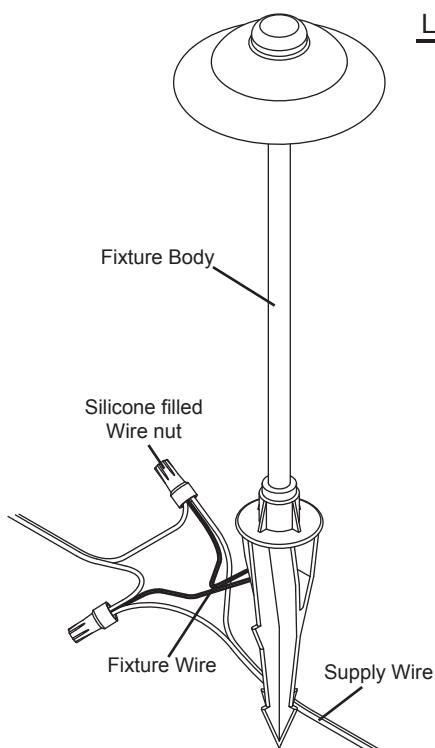
Note: Wire is to be protected by routing in close proximity to the Luminaire or fitting or next to a building structure such as a house or deck. Wiring should be buried a maximum of 6 inches (15.2cm) in order to connect to main supply wire. The main supply wire must have its length cut off within 6 inches (15.2cm) from a building structure, a Luminaire or fitting.
