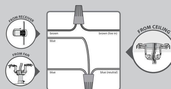
**CONNECT WIRES FROM RECEIVER AND FAN TO WIRES FROM OUTLET BOX** - Using the wire connectors, connect the brown (live in) wire from the ceiling to the brown wire from the receiver. Connect the blue (neutral) wire from the ceiling to both the blue wire from the receiver and the blue wire from the fan.
