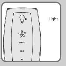
Quickly press the Light button to turn the lights off and on. Hold the Light button to raise and dim the light level.
