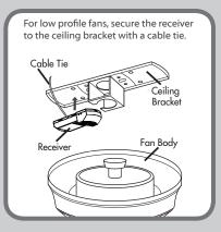
Choose the hanging system that most closely resembles the one used by your fan and install the receiver as shown and wire as directed.
