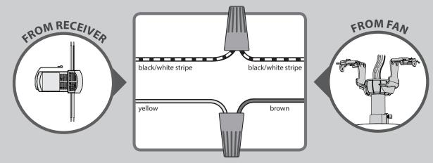
**CONNECT WIRES FROM RECEIVER TO FAN** - Using the wire connectors, connect the black and white wire from the receiver to the black and white wire from the fan. Connect the yellow wire from the receiver to the brown wire from the fan.
