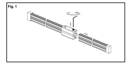
1. Unscrew the Allen Set Screws using the Allen Wrench provided.
