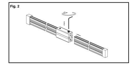
2. Insert the ends of the Rail firmly into the Rail Joiners and then tighten the Allen Set Screws.
