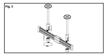
3. Remove the Standoff Caps. Slide the Rail into the Standoff. While supporting the Rail, screw the Standoff Caps back onto each of the Standoffs.
