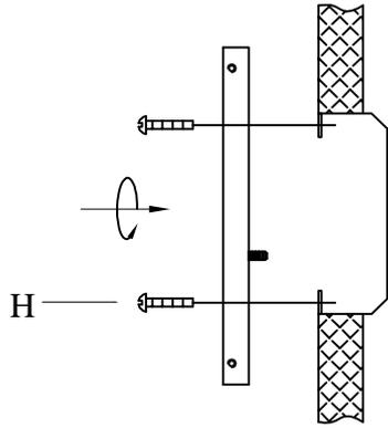
1. This step requires removing the mounting plate from the fixture.
