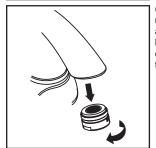
(4) Important: After installation is complete, remove the aerator. Turn on the water and allow both hot and cold water to run for at least one minute each. While water is running, check for leaks. Turn off the water and replace the aerator when finished.
