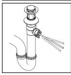
(6) Push pivot rod down and insert drain plug carefully. Test to ensure drain plug works properly.
