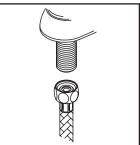
(3) When using stainless steel braided faucet supply hose, this faucet requires one end of the supply hose to have a 1/2" female IPS connection. The other end of this supply hose must match the thread on the water supply valve under your sink. Once you've identified the required size, carefully follow the manufacturer's installation instructions for each hose.
