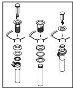
(2) a. For brass pop-up: Place a ring of plumbers putty on the bottom of the flange and apply Teflon tape on threaded tailpiece. Thread tailpiece to drain body. Insert flange through drain hole and attach drain body to flange from underneath the sink.
