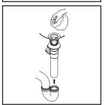
(4) Connect pop-up tail piece to the trap (check manufacturer's instruction for installation) and remove the excess plumbers putty.
