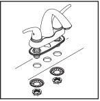
(2) Place the faucet in position on the sink. Apply plumbers putty under the base gasket. Install washer on shanks and tighten with locknut from under the sink
