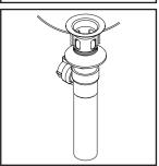
(3) Ensure the pivot rod hole on the pop-up body faces toward the back of the sink. Tighten the lock nut securely with a wrench.
