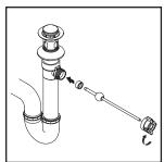
(5) Remove pivot rod nut from pop-up body and ensure the washer is in place. Insert pivot rod and tighten rod nut back to pop-up body.
