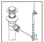
(7) Connect lift rod strap to pivot rod by using clip. Tighten thumbscrew to connect lift rod strap to pop-up lift rod.
