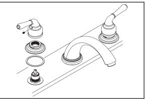
(3) Thread valve escutcheon with gasket onto valve, install lever handle on valve and tighten Allen screw with help of supplied Allen wrench. Install the other side of valve escutcheon and lever handle in the same way. Remove streamer, turn on handles to run water for one minute, check any leaks, replace streamer.
