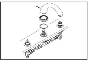
(2) Remove shank's test plug. Place spout escutcheon with gasket over top of shank. Carefully insert spout onto shank to avoid damaging O-rings on the shank. Make sure spout and spout escutcheon rest properly on finished surface. Secure spout by tightening Allen screw using supplied Allen wrench. Place button over Allen screw hole.
