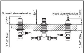
(1) Remove the guards, make necessary adjustment if the top of the shank and the tip of stem above finished surface do not follow the required heights. For deck thickness is equal to or less than 1-1/8", you don't need to use stem extension
