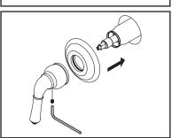
(3) Slide the flange on the sleeve against the finished wall. Apply silicone to caulk around the flange to form water tight seal. Attach the handle to the handle adapter. Tighten the Allen screw to secure the handle by using 3/32" Allen wrench. Check if the water diverts to desired outlet properly.
