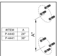
(1) Locate where to install the slide/grab bar and use a pen to mark the location of all six mounting screws. Use a power drill to drill 5/16" screw holes. Insert the screw anchors into the holes and hammer them flush to the wall as shown in the drawing.
