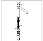
(2) Make sure washer is under escutcheon. Insert faucet through mounting hole. Tighten locknut to the faucet from underneath the sink with help of supplied mounting tool. Go to step (5) if faucet is without side spray.
