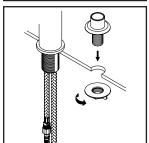
(3) For faucet with side spray, place side spray holder on mounting hole. Tighten locknut from underneath the sink to secure side spray holder.
