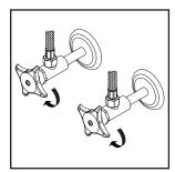
(1) Shut off the water supply. Remove old faucet. Clean mounting surface in preparation for new faucet.
