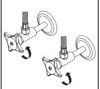
(6) Connect hot and cold inlet supply hoses to supply stops. For 1/2" connection; use 3/8" male to 1/2" female adapter for installation. Adapters are optional and not provided with the faucet. Turn on both sides of the supply
