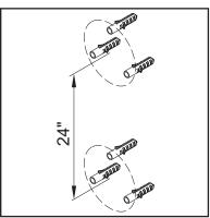
(1) Locate where to install the slide/grab bar and use a pen to mark the location of all six mounting screws. Use a power drill to drill 5/16" screw holes. Insert the screw anchors into the holes and hammer them flush to the wall as shown in the drawing.
