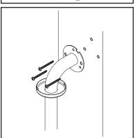
(2) Secure the slide/grab bar on the wall by tightening the mounting screws into the screw anchors. Place both flanges to cover the mounting screws as shown in the drawing.
