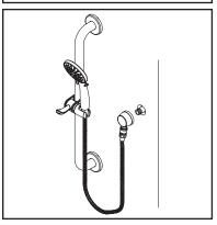
(3) Apply Teflon tape on the thread end of the pipe nipple and attach the drop ell to the pipe nipple. Connect the handheld shower and vacuum breaker to the hose and attach the hose to the drop ell. Turn on the water to check for any leaks.
