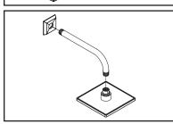
(3) Remove temporary nipple from the shower elbow. Use silicon to caulk the back of the shower arm flange. Slide the shower arm flange over the shower arm. Apply the Teflon tape on the both threaded ends of shower arm and install the shower arm to the shower elbow. Carefully tighten with a clean strap wrench. Press the shower arm flange against the finished wall. Flush out the system. Thread the showerhead to the shower arm.
