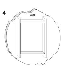
Carefully complete the frame with studs and frame blocks inside the cutout, making sure that edges align.
