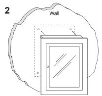
With a level, position your medicine cabinet to your desired wall location. Align and drill holes into the wall that matches the drilled holes of your medicine cabinet. Secure your medicine cabinet using four Hollow Wall Anchors.
