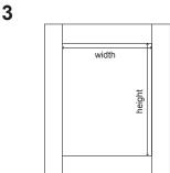
Create a frame using frame studs and frame blocks that would fit the width and height of the backside of your medicine cabinet.
