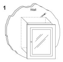
Using a pencil and a level draw the perimeter of the backside of the cabinet in desired wall location.
