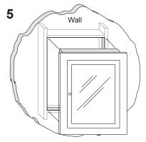
Place an appropriate amount of wood glue on the inner sides of the frame. Position the cabinet into the cutout and into the frame.
