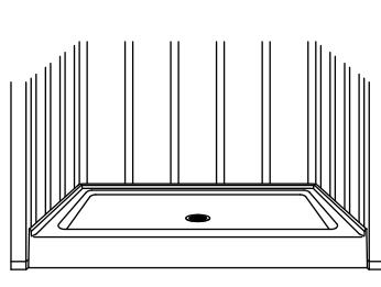
**7** With the unit level, shim under the support feet as needed.
