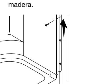
**17** Secure the walls to the studs along the top. Use shims as needed.
