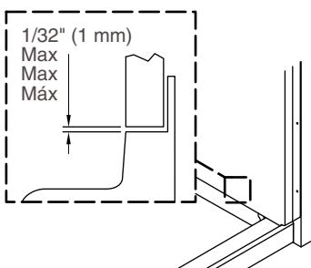
**16** Starting at the bottom, install screws through the dimples to secure the flanges to the studs.
