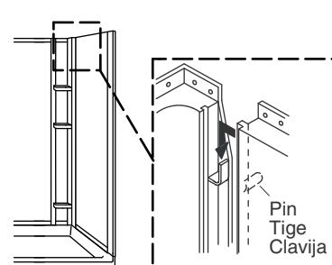
**15** The front edges should be flush, with no more than a 1/32" (1 mm) gap.
