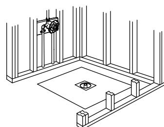
**5** Without a pad, we recommend the basin area be set in 1" (25 mm) to 2" (51 mm) of mortar cement.
