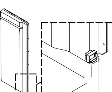
**14** Install the end walls. Engage the end wall pins in the back wall slots.
